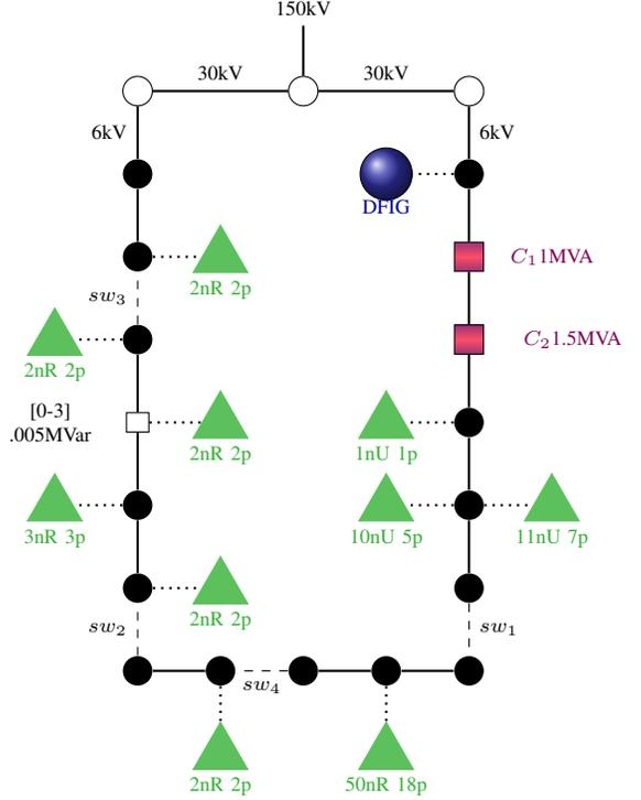
Fig. 2: Network example. Ring topology with 20 buses, plus another 85 buses in tree subnets fed from the main loop, indicated by triangles: label  $XnY Zp$  where  $X$  is # of buses,  $Y$  the type (rural or urban) and  $Z$  the tree depth. Squares indicate buses with industrial loads (right) and capacitor bank (left). Relevant switches are dashed lines.
