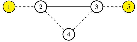
Fig. 1: Example network. Substations are nodes 1 and 5. Dashed lines have switches.
